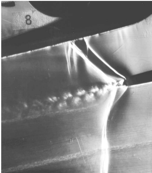
Fig. 11 Shedding of doublets at Ma=1.07
